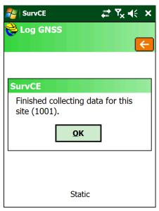
When you have completed the last occupation, close the file by click-holding the Files button on the receiver for 2-seconds.
