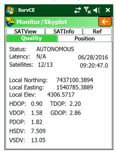
If you have a position, and the Yellow LED is flashing then there is a file open, you are connected and you are ready to collect raw data.
