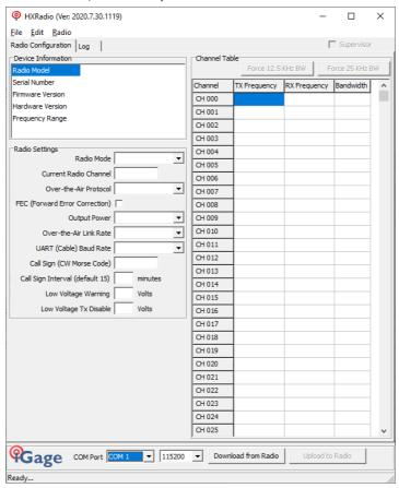
Begin by attaching the radio to a serial port and powering the radio on. After the radio boots, make sure the selected 'COM Port' matches the COM port the radio is connected to:
