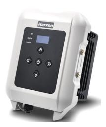
This manual is for use with Harxon DU8616 35-Watt digital radio supplied by iGage Mapping Corporation. Radios purchased from other sources cannot be programmed without an iG key code which is only available for iGage supplied devices.
