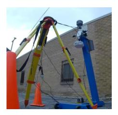
systematically dumps 1 to 4 GNSS receivers and records the subsequent Time-to-Fix and range of FIXED measurements for each receiver under test. Dumps are achieved by physically rotating the receiver upside down and then rotating it back to face skywards.
