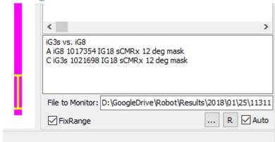
The lower right corner of the plot screen allows the operator to pick a test result to display. Results for all devices under test are kept in a file named 'GPS\_ALL.log' in the test folder (folders are automatically generated for each test using '../YYYY/MM/DD/HHMMSS/' format under a master result folder.
