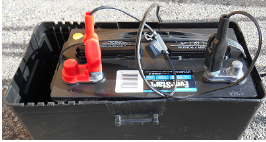
Figure 11 Alligator-clip connections won't support full output power!
